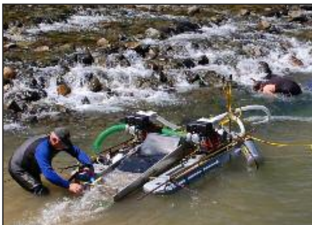
The picture above shows a typical dredging operation with our new 6218 HM 6 inch dredge featuring the new HP500 pump.
