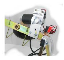
Attach the motor / switch plate to the cross member using the bolts and washers provided.
