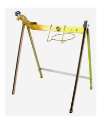
The assembled legs and cross member should look like this with the wire hanger for the gold pan attached to the crossmember.
